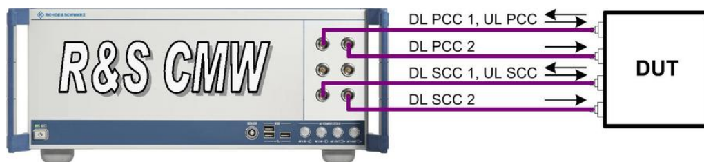
Figure 2-5: Test setup for CA, four DL, two UL, 4 DUT antenna connectors
