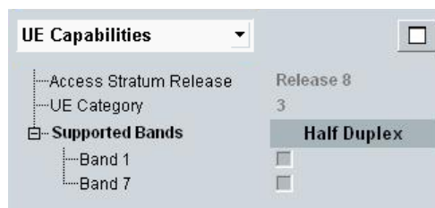
Figure 2-41: UE capabilities in the main view
