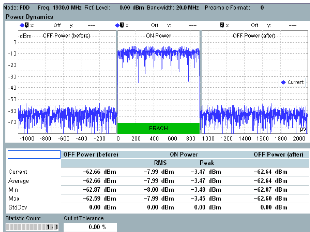
Figure 4-11: LTE PRACH: Power Dynamics
