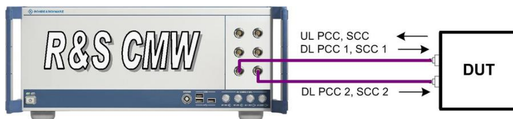
Figure 2-4: Test setup for CA, four DL, two UL, 2 DUT antenna connectors
